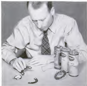
Cut the magnetized ring, and the parts have poles
